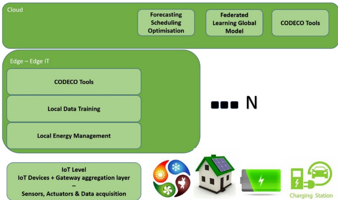
Figure 37: P4 system architecture
