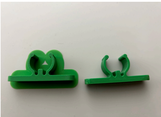
Figure 24: Faulty(left), non-faulty objects.
