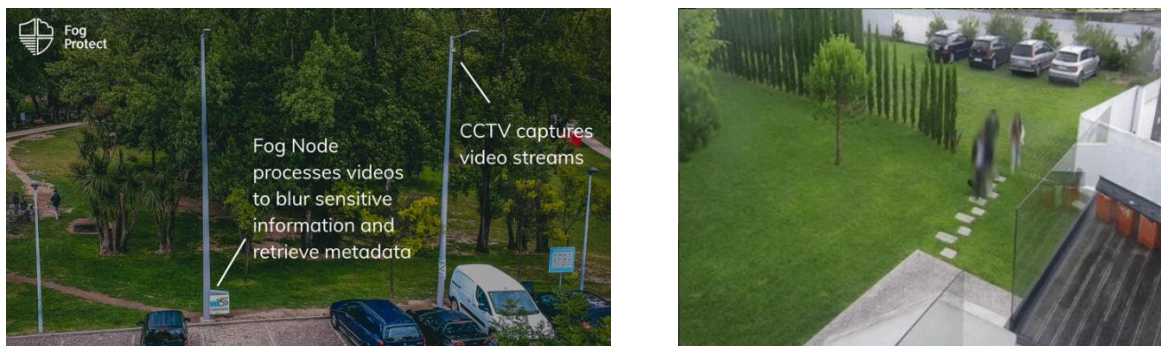
Figure 8: Schematic depiction of the smart cities use case deployment (left), video frame sample from the fog node after blurring sensitive data (right).
